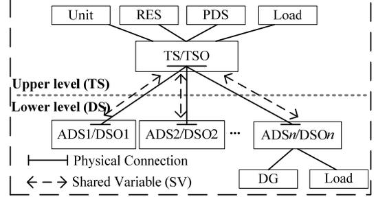
Fig. 1. Structure of the TS-DSs restoration system.
