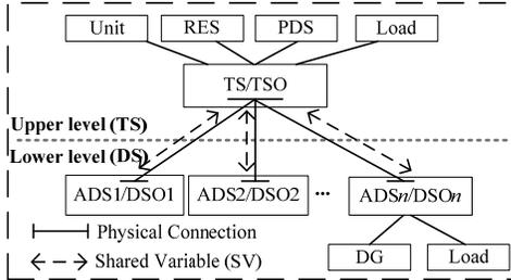
Fig. 1. Structure of the TS-DSs restoration system.
