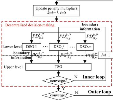
Fig. 4. ATC based iterative process of TS-DS interaction
