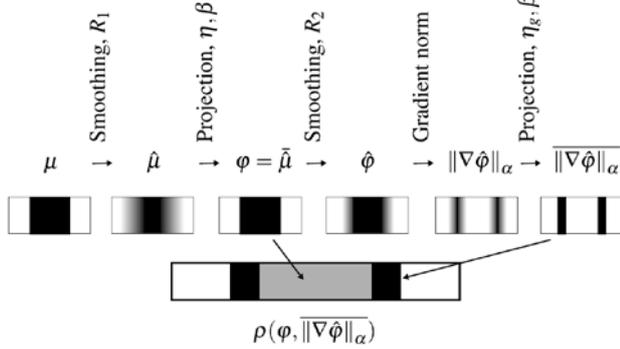
**Figure 1.** Illustration of the filter hierarchy used for the coating design approach. Image taken from [3].
