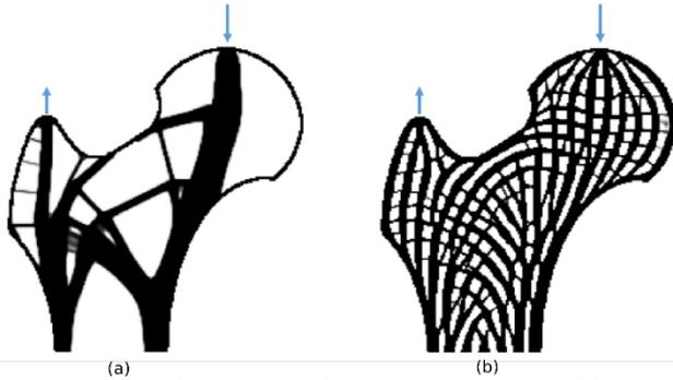
**Figure 2.** Result of standard TO (a) and the infill method (b) using a single load case. Image from [5].
