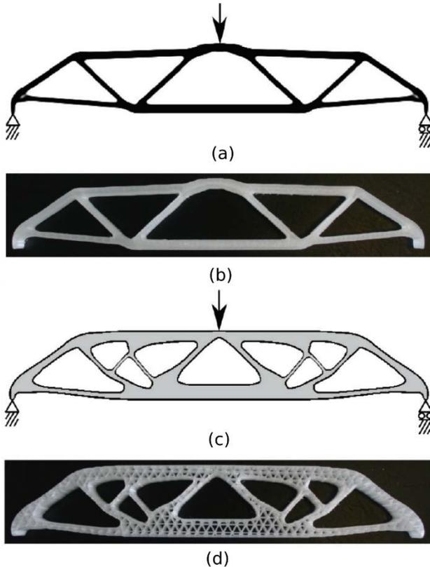
**Figure 2.** Result of standard TO (a) and an FDM printed specimen (b). Image (c) shows the result using the coating approach and its FDM specimen in (d). Image from [4].
