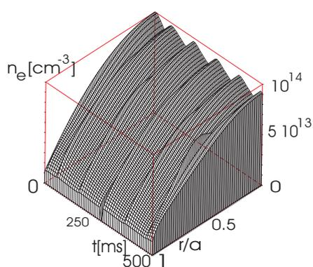
Fig.5 Time evolution of the density  $N_e$  with repetitive pellet injection
