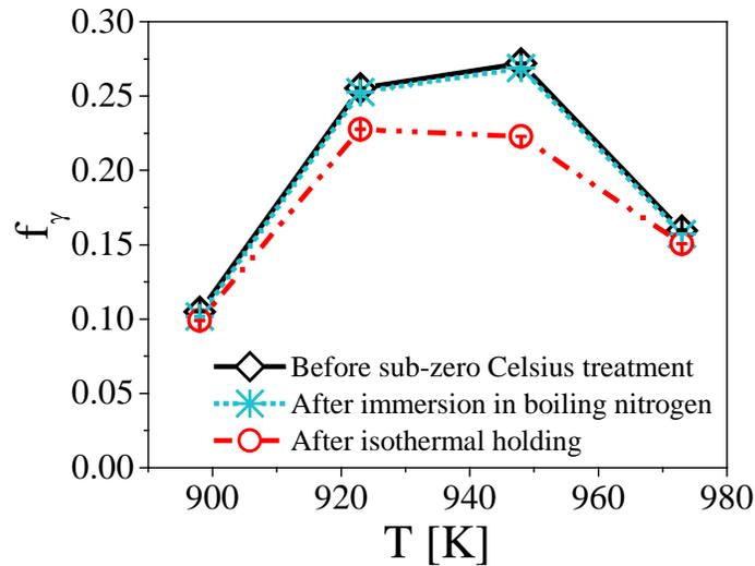
**Figure 2. Fraction of austenite  $f_{\gamma}$  versus annealing temperature T. The three data sets refer to the material before sub-zero Celsius treatment, after immersion in boiling N<sub>2</sub> for 0.3 ks and after additional isothermal holding at 195 K for 15.3 ks.**
