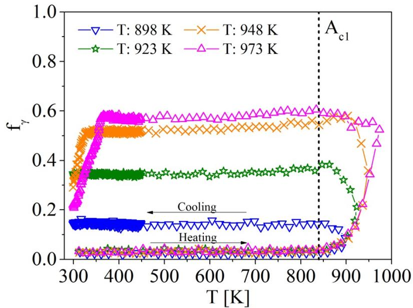
**Figure 1. Fraction of austenite  $f_\gamma$  versus temperature  $T$  for four inter-critical annealing treatments. Numbers in the legend refer to the temperature reached during the heating step, immediately followed by cooling.**
