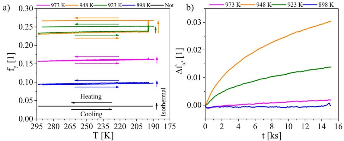
**Figure 4. VSM results from of sub-zero Celsius treatment: (a) Fraction of austenite,  $f_\gamma$ , of the differently tempered samples vs. temperature for cooling to 195 K with  $0.25 \text{ K.s}^{-1}$ , isothermal holding for 15.3 ks and reheating to room temperature with  $0.25 \text{ K.s}^{-1}$ ; (b) Fraction transformed,  $\Delta f_{\alpha'}$ , vs. time during isothermal holding at 195 K.**
