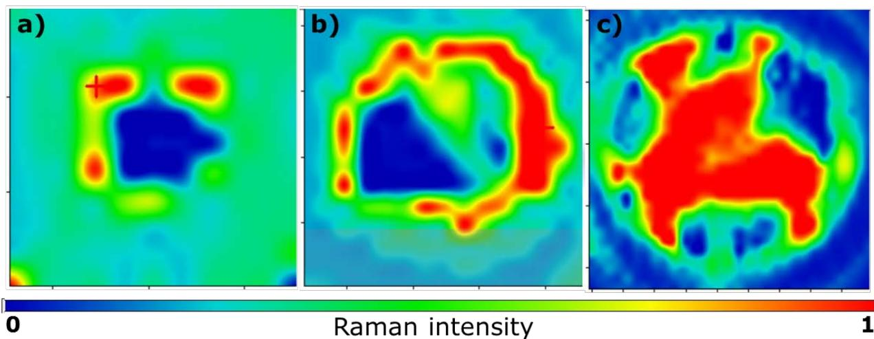
**Fig. 2:** Raman map on peak 1003 cm<sup>-1</sup> representing the distribution of ketoprofen in the uppermost layers inside the of a) small, b) medium and c) large MCs.
