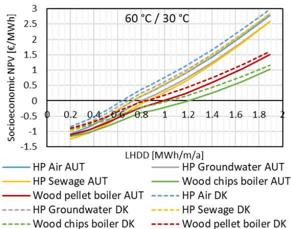
Figure 3 socioeconomic NPV for DK and AUT, DH temperatures of 60 °C/ 30°C, NB medium, lin. cost function
