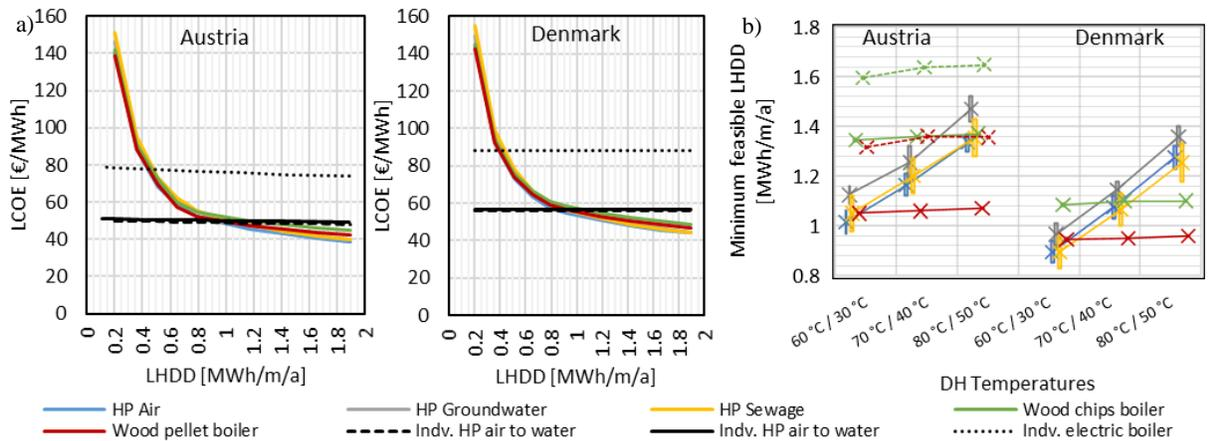
Figure 2 a) LCOE for central and individual units for Austria and Denmark, DH temperatures of 60/30 °C, NB-medium and linear HP cost functions , b) Range of minimum feasible LHDD for central solutions for different DH temperature cases, dashed lines refer to cases without subsidies
