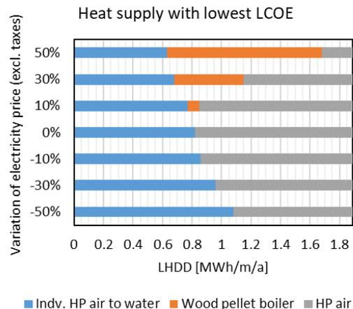
Figure 4 Solution with lowest LCOE for varying LHDD and electricity price, DH temperatures of 60 °C/ 30°C, NB medium, lin. cost function
