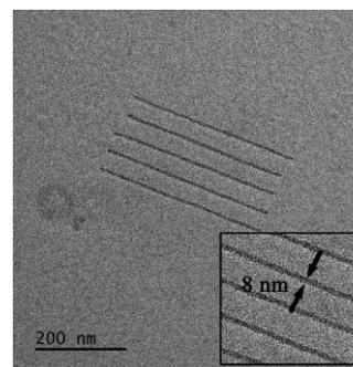
Figure 3. Patterned undecane (C<sub>11</sub>H<sub>24</sub>) lines with average line widths of 8 ± 1 nm.
