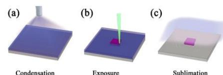
Figure 1. Basic implementation of organic ice lithography. (a) A vapor of organic precursor condenses on a substrate cooled down to cryogenic temperature. (b) During e-beam exposure, the chemical structure of the exposed area is altered resulting in the formation of a non-volatile product. (c) After heating the substrate to a room temperature, the unexposed resist sublimates, while the exposed area remains.
