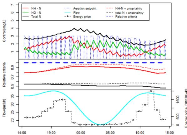
Fig. 1. Upper: Example of optimal aeration signal and the expected development in  $NH_4$ ,  $NO_3$  and total-N. Middle: Relative criteria compared to legislative requirements. Bottom: Predicted inflow and Electricity prices from day-ahead-market
