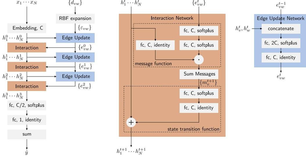
Figure 1: Flow of computations of the proposed model. The dimension of the hidden state for each atom state is  $C$  and the “fc”-blocks are fully connected layers annotated with the output dimension and the applied activation function.
