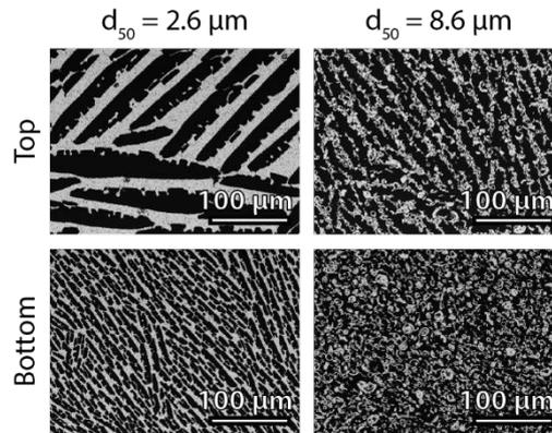
**Figure 4: SEM images of cross sections perpendicular to the freezing front obtained at the top (sample height: 18 mm) and bottom (sample height: 4 mm) of samples prepared from ceramics of various particle size.  $d_{50}$  denote the median particle size of the particle size distribution of freeze-casted suspensions.**
