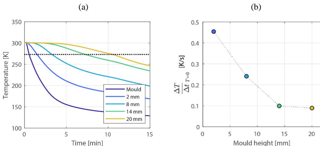
**Figure 3: Freezing conditions for freeze-casted LCSM ceramics. (a) Temperature of mould bottom and at various positions along the height of the mould, the freezing point of water is indicated by the dashed line, and (b) the local freezing rates at the time of freezing.**
