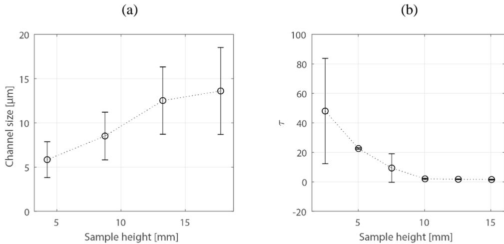
**Figure 2: Structural properties of freeze-casted LCSM ceramics. (a) Channel size is measured as the width of lamellar pores on SEM images of perpendicular cross sections at various sample heights, while (b) tortuosity is calculated from SEM images obtained at various heights parallel to the freezing direction.**
