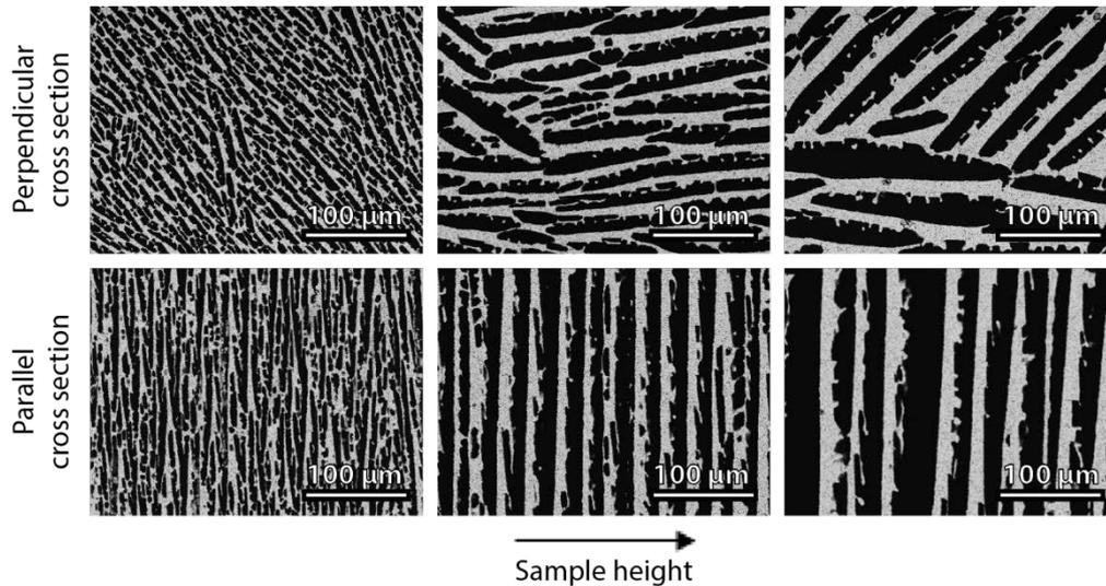
**Figure 1: SEM images of cross sections perpendicular and parallel to the freezing direction, where the grey parts are ceramic walls while the black areas are voids or channels. Directional freezing thus results in a hierarchical, porous structure of lamellar micro-channels.**
