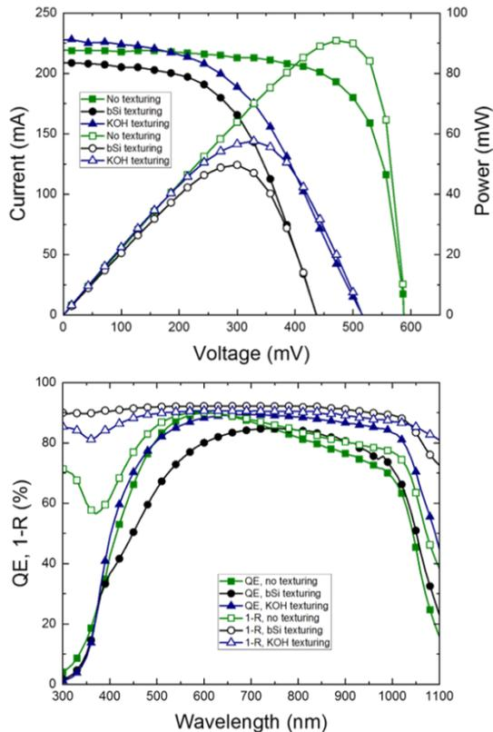
**Figure 5:** Characterization of solar cells with different surface texturing. Top: current-voltage characteristics under 1 Sun illumination. Bottom: quantum efficiency and front surface reflection subtracted from unity as function of photon wavelength.
