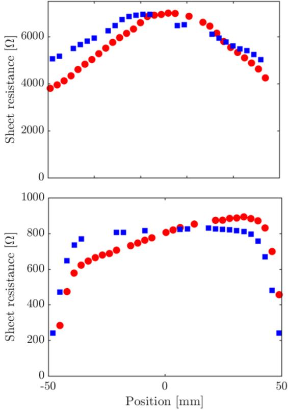
**Figure 2:** Sheet resistance measured along two perpendicular directions across a planar 100 mm wafer for p-type poly-Si (top) and n-type poly Si (bottom). Thickness of the poly-Si is 40 nm for both wafers.
