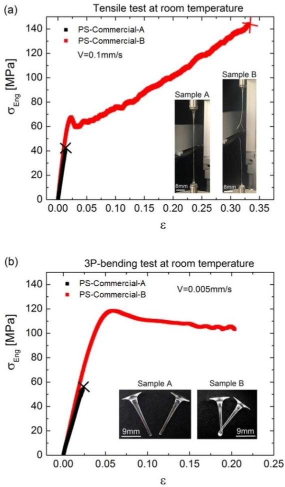
**Figure 1.** Engineering stress as a function of strain in (a) tensile tests, and (b) 3-point bending tests, at room temperature for PS-Commercial. Sample A is isotropic, while Sample B is an anisotropic sample with molecular alignment. The crosses represent the fracture points.
