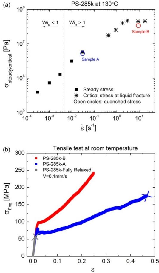
**Figure 2.** (a) Steady stress (taken from Ref. [17]) and critical stress at fracture as a function of stretch rate for PS-285k at 130°C. The Weissenberg number is defined as  $Wi_R = \dot{\epsilon}\tau_R$ . (b) Engineering stress as a function of strain at room temperature for the quenched PS-285k samples.
