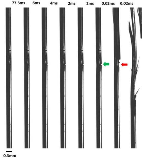
**Figure 4.** High-speed images taken at 50,000 frames per second showing the fracture process for PS-Commercial-B in the tensile test. The time between the adjacent frames are shown on the top. The green arrow marks a small crack with an approximate parabolic outline, and the red arrow shows that it changes to a sliding pattern.
