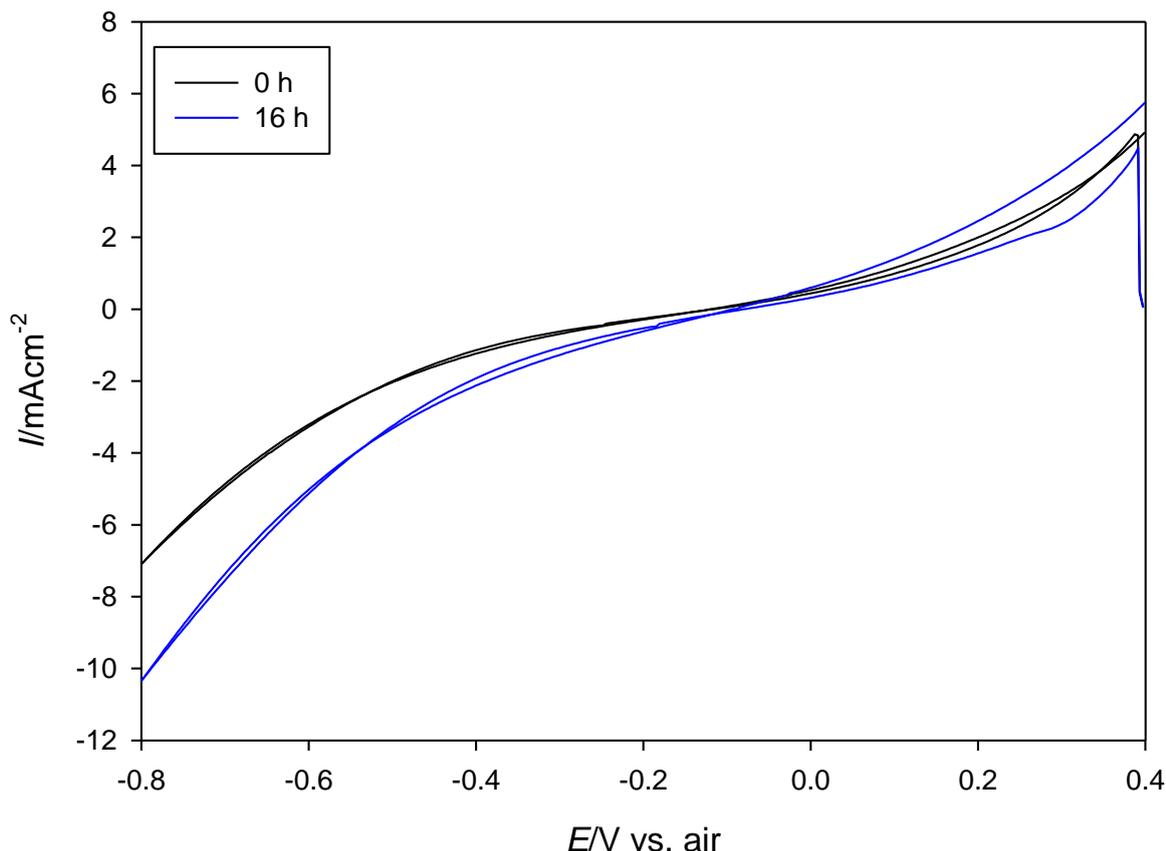
**Figure 7.** Voltammograms recorded for LSM50 in 1% nitric oxide in argon at 400 °C with a sweep rate of 10 mV/s. The solid curve was recorded without anodic pretreatment, whereas the dotted curve was pretreated at a potential of 0.4 V vs. air for 16 h. The magnitude of the current densities is highest for the LSM00 electrode treated at 0.4 V vs. air before recording the voltammogram.
