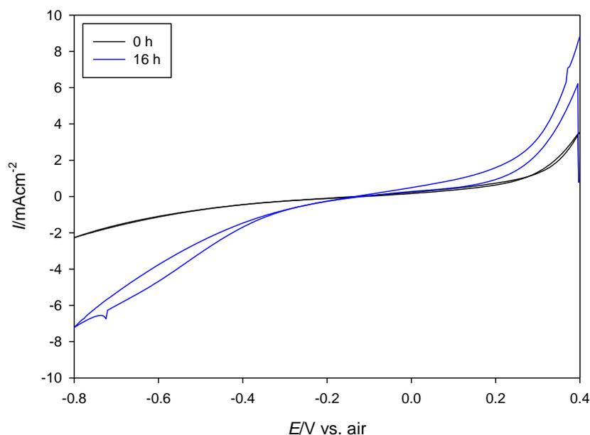
**Figure 5.** Voltammograms recorded for LSM15 in 1% nitric oxide in argon at 400 °C with a sweep rate of 10 mV/s. The solid curve was recorded without anodic pretreatment, whereas the dotted curve was pretreated at a potential of 0.4 V vs. air for 16 h. The magnitude of the current densities is highest for the LSM00 electrode treated at 0.4 V vs. air before recording the voltammogram.
