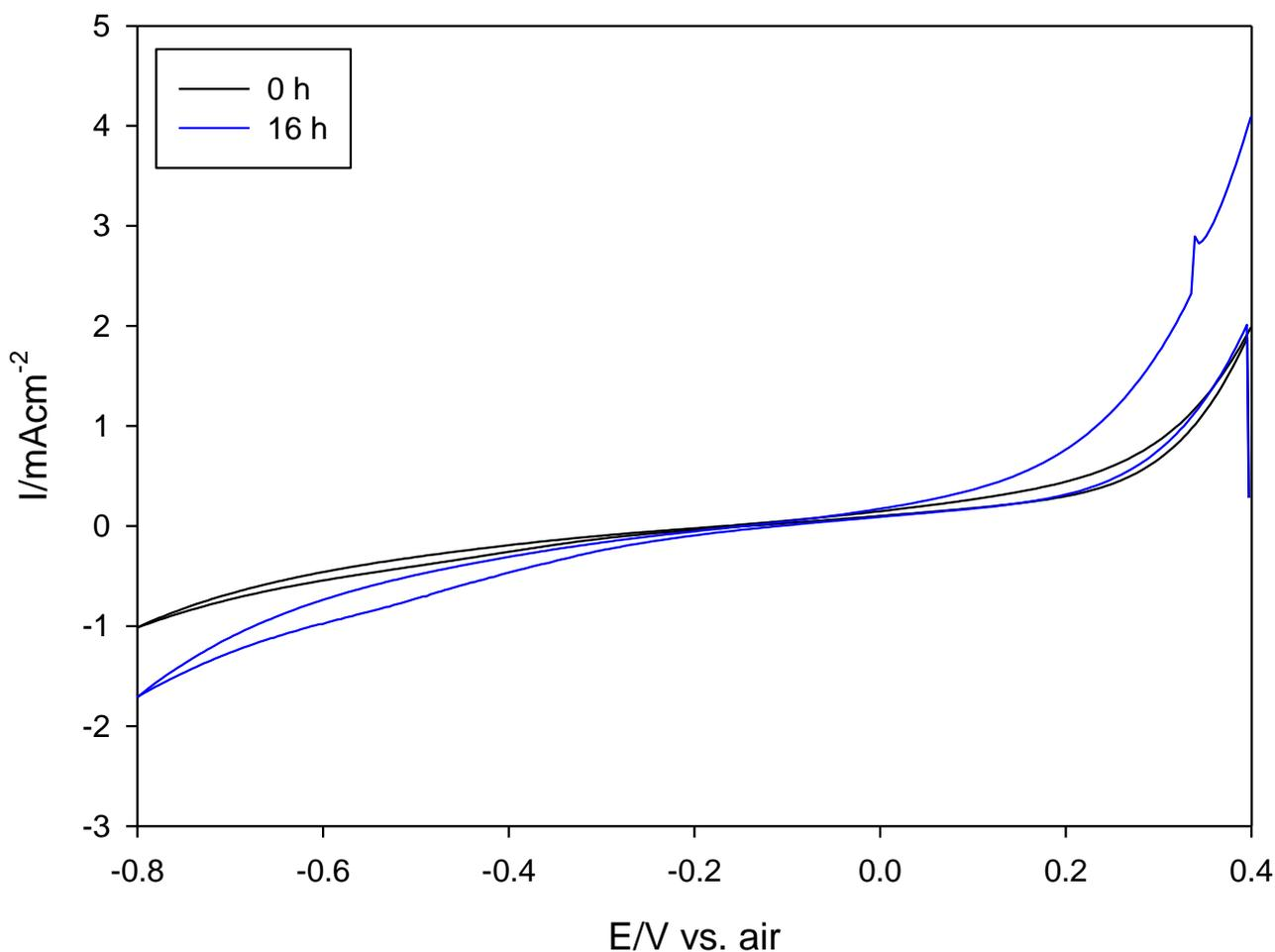
**Figure 3.** Voltammograms recorded for LSM00 in 1% nitric oxide in argon at 400 °C with a sweep rate of 10 mV/s. The solid curve was recorded without anodic pretreatment, whereas the dotted curve was pretreated at a potential of 0.4 V vs. air for 16 h. The magnitude of the current densities is highest for the LSM00 electrode treated at 0.4 V vs. air before recording the voltammogram.
