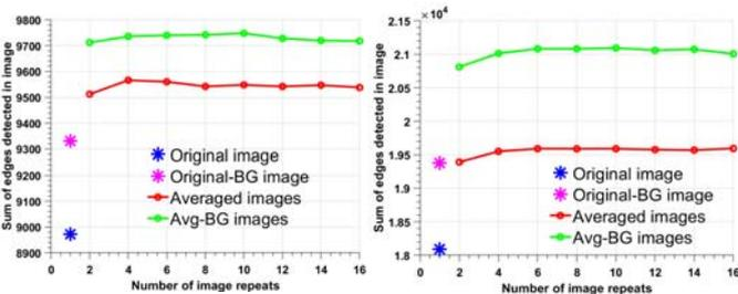
Fig. 11 Graph displaying effect of number of repeats on the edge detection technique used in the EL measurement for (i) Original (ii) Averaged (iii) Original-BG and (iii) Avg-BG images. Left side graph is imaged by camera 1 and right side graph by camera 2 for Panel B.
