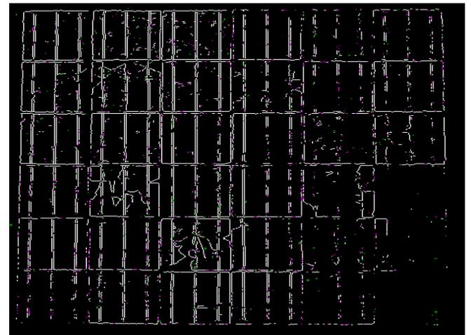
Fig. 14 Overlapping of Original and Averaged-Background images for Panel B imaged with camera 1. The difference in the sum of edges detected can be seen by the red-cyan color in the image.
