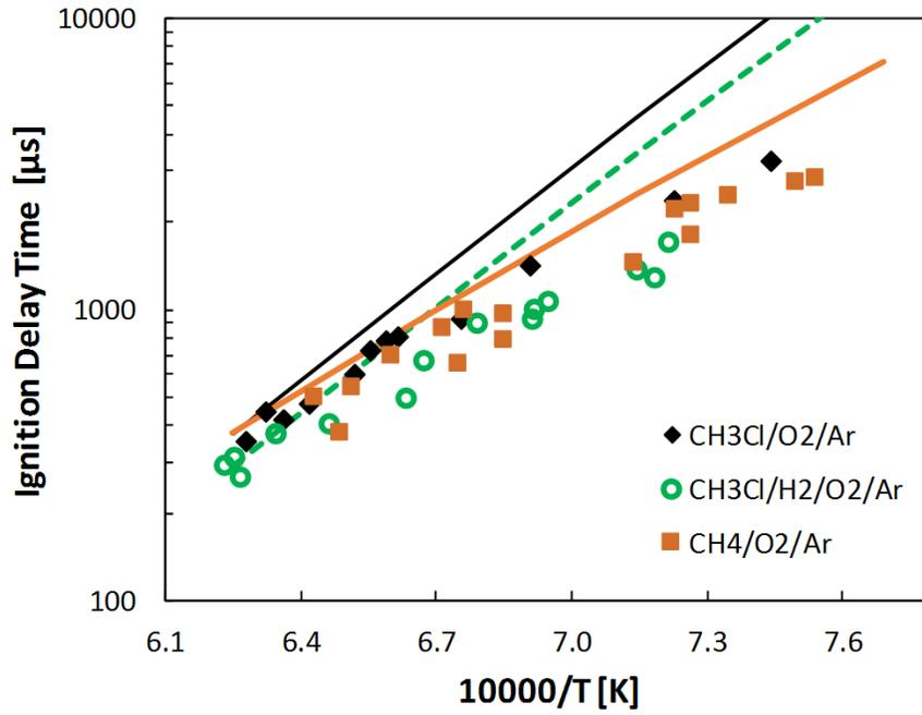
Figure 9: Ignition delay times for CH<sub>3</sub>Cl, CH<sub>4</sub>, and a CH<sub>3</sub>Cl/H<sub>2</sub> mixture. Symbols mark experimental results from Miller et al.<sup>17</sup> and lines denotes the prediction of the present model. The pressure behind the reflected shock was 2 atm. Inlet compositions: 10% CH<sub>3</sub>Cl and 15% O<sub>2</sub> (mixture 1); 10% CH<sub>4</sub>, 15% O<sub>2</sub> (mixture 2); 10% CH<sub>3</sub>Cl, 1% H<sub>2</sub>, 15% O<sub>2</sub> (mixture 3); balance Ar.
