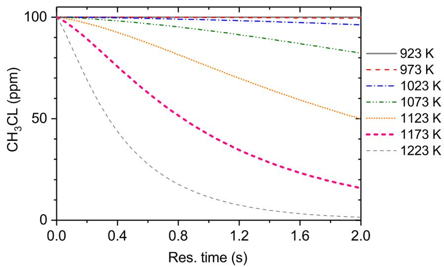
Figure 12: Thermal conversion of methyl chloride within a CFB gasifier. The initial gas composition for the simulation is 11% H<sub>2</sub>, 14% CO, 16% CO<sub>2</sub>, 6.2% CH<sub>4</sub>, 1.6% C<sub>2</sub>H<sub>4</sub>, 12% H<sub>2</sub>O; balance N<sub>2</sub> (see Table 2). The pressure is atmospheric; temperature and residence time as shown in the figure.
