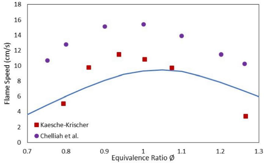
Figure 10: Laminar burning velocities of methyl chloride-air mixtures as a function of fuel-air equivalence ratio. The squares are experimental results from Kaesche-Krischer<sup>62</sup> while the circles are from Chelliah et al.<sup>24</sup> The line denotes the model predictions. The initial temperature was 298 K while the pressure was 1 atm.
