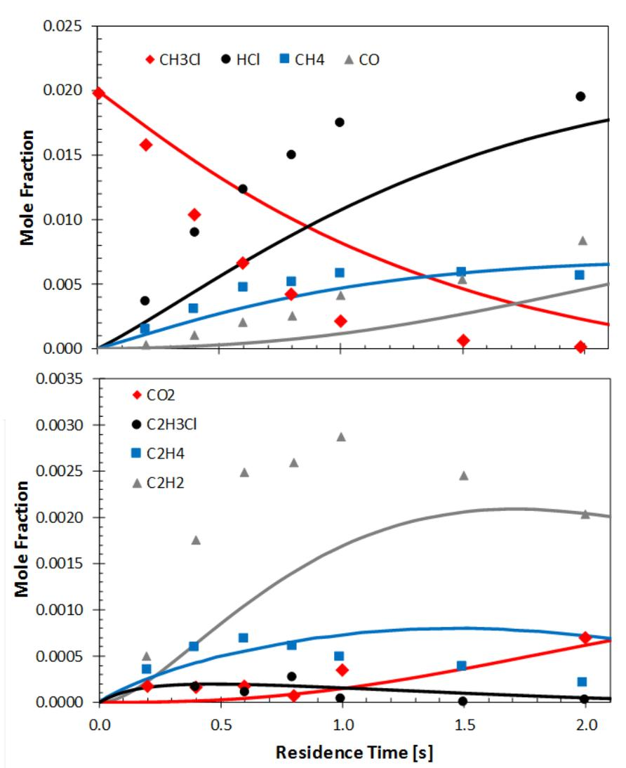
Figure 8: Comparison of experimental data (symbols) and model prediction (lines) for the oxidation of methyl chloride in a  $\text{H}_2/\text{O}_2/\text{Ar}$  mixture plotted as a function of residence time for a fixed temperature of 1173 K. The initial concentrations were 1%  $\text{H}_2$ , 1%  $\text{O}_2$ , 2%  $\text{CH}_3\text{Cl}$  and 96% Ar. The experiments were conducted at 1 atm and the experimental results are from Ho et al.<sup>13</sup>
