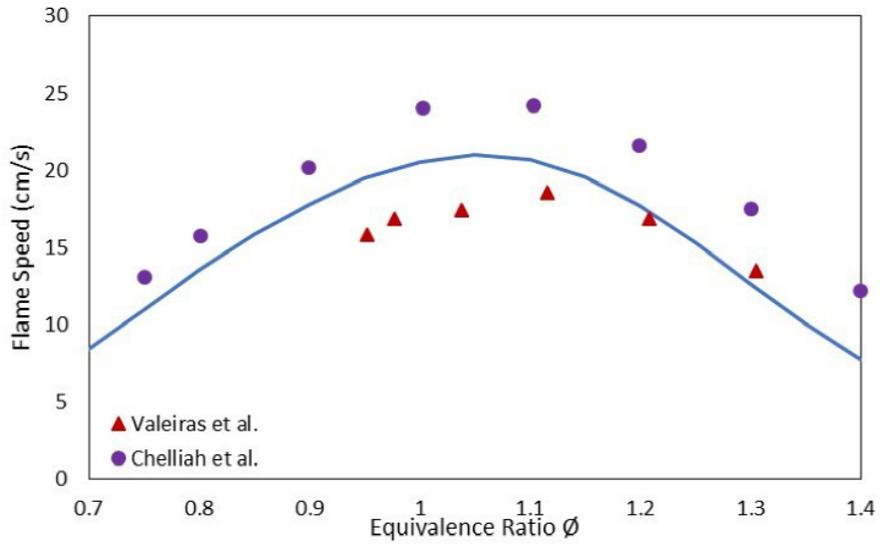
Figure 11: Laminar burning velocity of fuel mixtures of 50%  $\text{CH}_3\text{Cl}$  and 50%  $\text{CH}_4$  in air as a function of fuel-air equivalence ratio. The experimental results are from Valeiras et al.<sup>22</sup> and Chelliah et al.<sup>24</sup> The initial temperature was 293-298 K while the pressure was 1 atm. The predictions were made for a temperature of 298 K.
