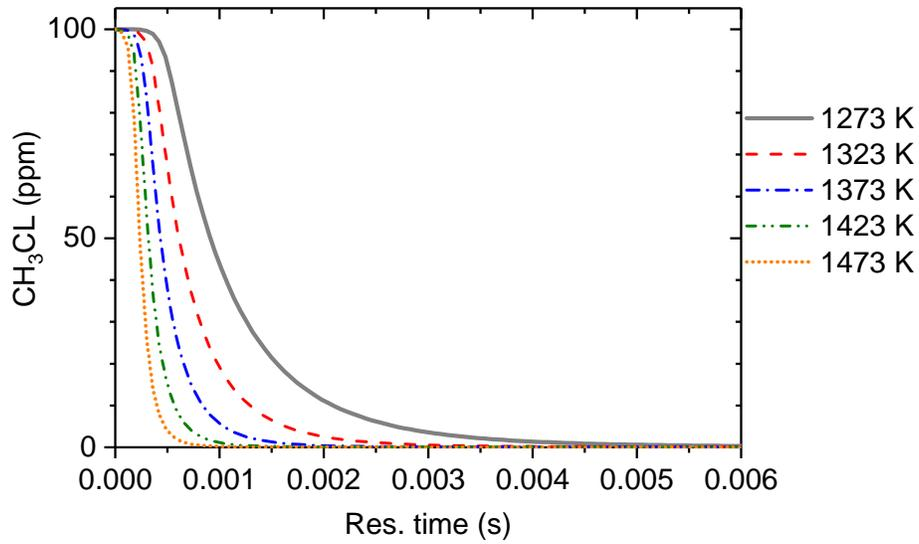
Figure 14: Thermal conversion of methyl chloride within a downdraft gasifier with 1% of oxygen present. The initial gas composition for the simulation is 20% H<sub>2</sub>, 21% CO, 14% CO<sub>2</sub>, 1.4% CH<sub>4</sub>, 1.0% O<sub>2</sub>; balance N<sub>2</sub> (see Table 4). The pressure is atmospheric; temperature and residence time as shown in the figure.
