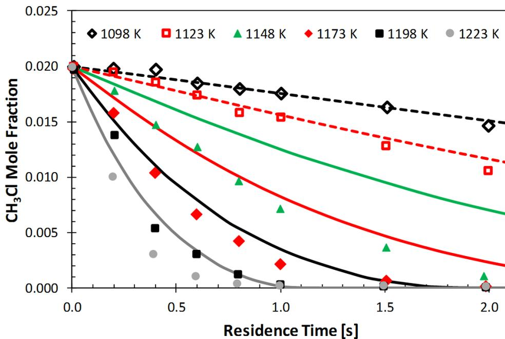
Figure 7: Comparison of experimental data (symbols) and model prediction (lines) for oxidation of methyl chloride in  $H_2/O_2/Ar$  mixtures at different temperatures. The initial concentrations were 1%  $H_2$ , 1%  $O_2$ , 2%  $CH_3Cl$  and 96% Ar. The experiments were conducted at 1 atm and the experimental results are from Ho et al.<sup>13</sup>
