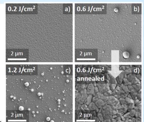
Fig. 4 Droplets on films at different fluence. No peaks detected in XRD, indicating the films and the droplets are amorphous
