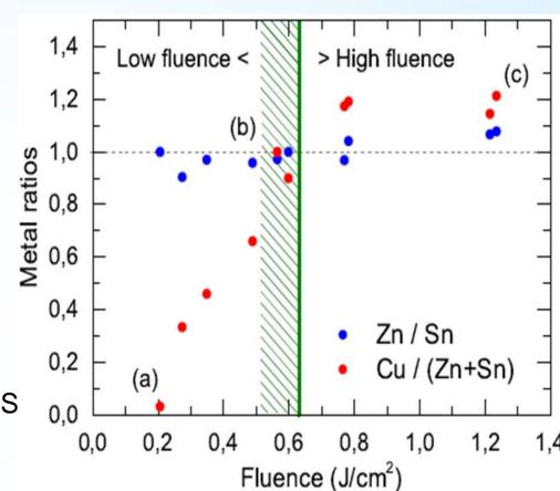
Fig. 3: Non-stoichiometric material transfer as function of laser fluence. Copper content varies significantly, while Zn and Sn are kept in stoichiometric proportion (within EDX detection limit, grey bar). S content not shown for clarity.
