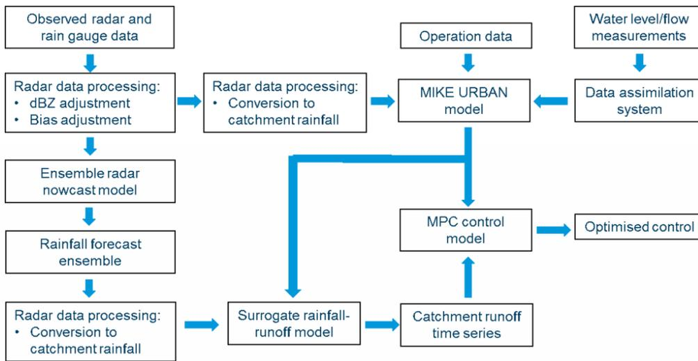
**Fig. 2.** Established workflow for the real-time control system
