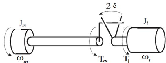
Fig. 2. Backlash: When the difference between the motor and the load position is smaller than  $\delta$ , then the two shafts are disengaged and no torque is applied to the motor or the load. The picture is taken from Nordin and Gutman [2002].
