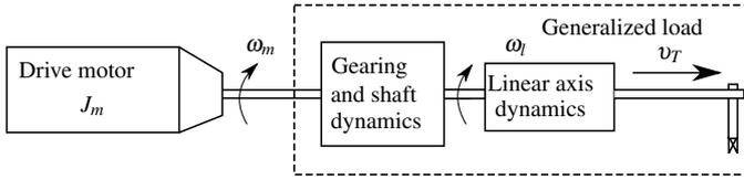
Fig. 1. Correspondence between mechanical drive-train and single-axis machine-tool systems. The angular velocities of the motor and the load are denoted by  $\omega_m, \omega_l$ , respectively, while  $v_T$  is the tool linear velocity.
