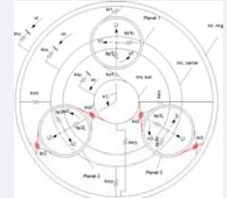
In case of a double contact the sun can be "caught" by two planets causing an uneven load distribution.
