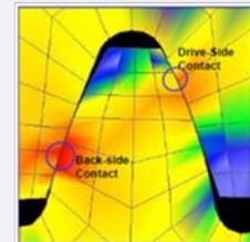
In case of large bearing clearance a double contact can occur, where the tooth backside is also in contact.
