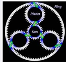
Load pattern during normal operation when loading is as expected with pressure on one tooth side only
