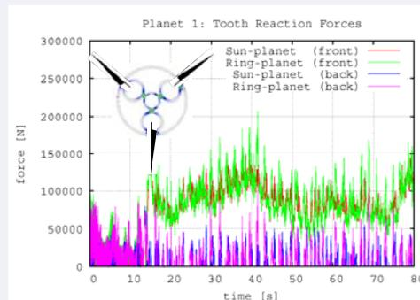
Large carrier bearing clearance is applied which causes double contact. Loads are increased significantly. The rotor is "mounted" so that the three planets are aligned with a blade.
