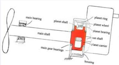
A traditional layout of the drive train is modeled where the gearbox also acts as the second main bearing. The rotor loads, weight and inertial forces of the gearbox are carried by the planet carrier.
