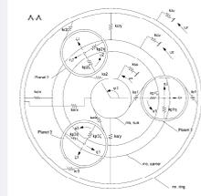
2-dimensional model of planetary gear stage with lumped springs representing tooth and bearing stiffness.
