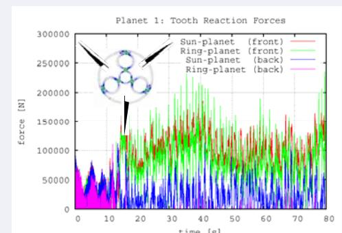
Same gearbox as the one to the left, but the "mounting" of the gearbox relative to the blades is rotated 60deg. This results in an even larger load increase.
