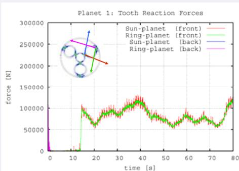
Normal operation case without double contact. The variation in loading is caused by turbulent wind speed variation. Tooth force directions are illustrated with arrows.
