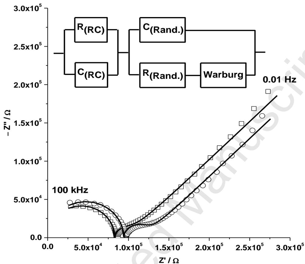
**Fig. 4.** Nyquist plots representing selected typical impedance response of the studied solid-contact ISEs together with the fit (solid lines), where □ is a  $Pb^{2+}$ -ISE conditioned in  $Pb(NO_3)_2$  (IV) and ○ is a  $Pb^{2+}$ -ISE conditioned in PBS, BSA and  $Pb(NO_3)_2$  (V). The numerals (IV) and (V) refer to **Scheme 1**. Insert: equivalent circuit used for fitting.
