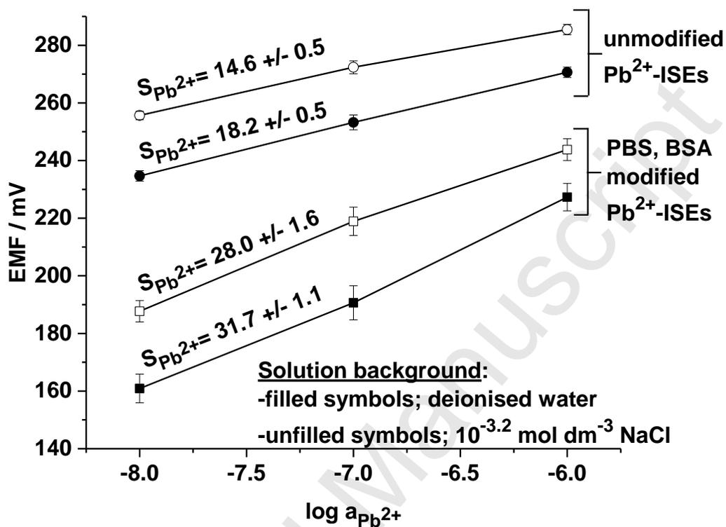
**Fig. 7.** Potentiometric response of unmodified (circles) and BSA and PBS modified (squares)  $Pb^{2+}$ -ISEs in standard solutions of  $Pb(NO_3)_2$  measured between  $10^{-8}$  and  $10^{-6} \text{ mol dm}^{-3} Pb^{2+}$  with various standard solution background, namely deionized water (filled symbols) and  $10^{-3.2} \text{ mol dm}^{-3} NaCl$  (unfilled symbols).
