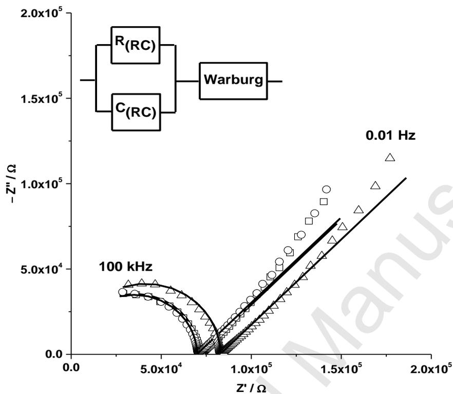
**Fig. 3.** Nyquist plots representing selected typical impedance response of the studied solid-contact Pb<sup>2+</sup>-ISEs together with the fit (solid lines), where  $\square$  is an unconditioned Pb<sup>2+</sup>-ISE (I),  $\circ$  is a Pb<sup>2+</sup>-ISE conditioned in PBS (II) and  $\Delta$  is a Pb<sup>2+</sup>-ISE electrode conditioned in PBS and BSA (III). The numerals (I)-(III) refer to **Scheme 1**. Insert: equivalent circuit used for fitting.
