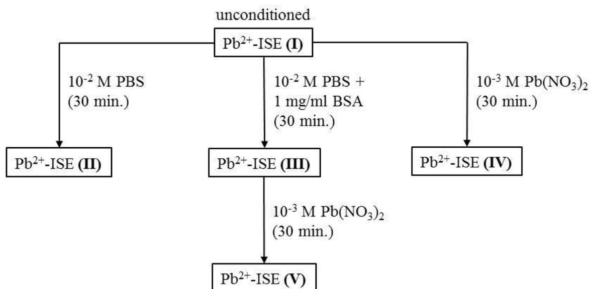
**Scheme 1.** Conditioning protocol for  $\text{Pb}^{2+}$ -ISEs (I) – (V).
