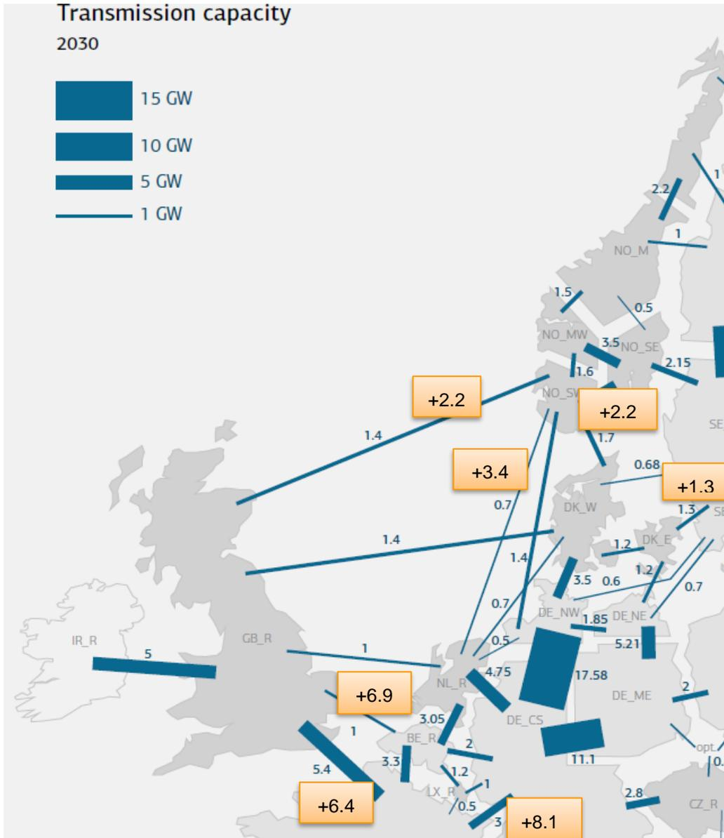
**Figure 7: Transmission capacity according to TYNDP 2014 [7] by 2030 (dark blue) and calculated capacity additions [1] (GW; orange fields) by 2050. The additions are also reported in the matrix in Table 1.**
