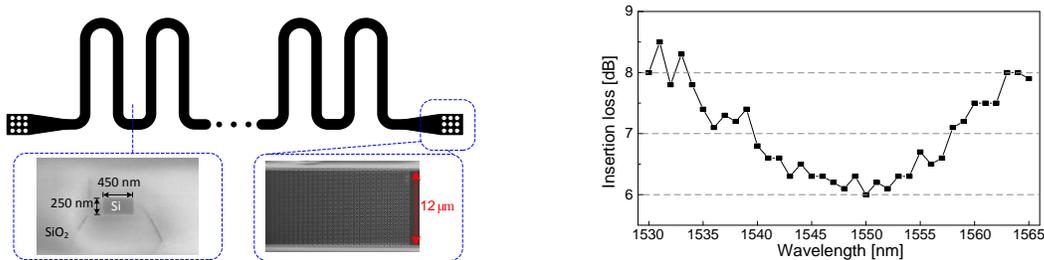
**Fig. 1** Left: Schematic of the Si-nanowire with grating couplers. The insets show a scanning electron microscopy (SEM) image of the cross-section of the Si-nanowire and the apodized PhC grating coupler. Right: Insertion loss of the grating coupled Si-nanowire including coupling loss and propagation loss.
