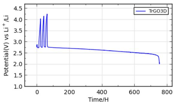
Figure 6: Battery test of a TrGO3D cathode tested at 0.1 mA/cm<sup>2</sup>.
