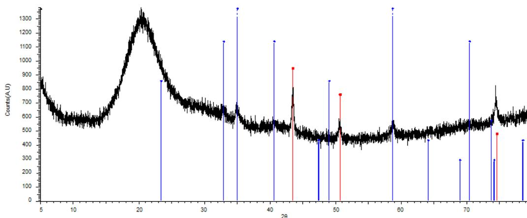
Figure 7: XRD of deep discharged TrGO30min battery cathode with peak assignment: blue =  $\text{Li}_2\text{O}_2$  and red = SS mesh, FeNi. The XRD diffractogram shows only reflections from crystalline  $\text{Li}_2\text{O}_2$  and no carbonate formation is observed.
