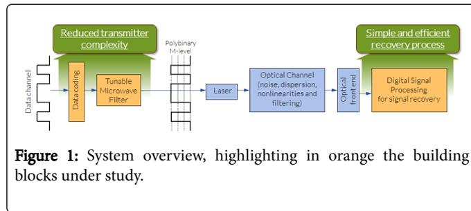
**Figure 1:** System overview, highlighting in orange the building blocks under study.
