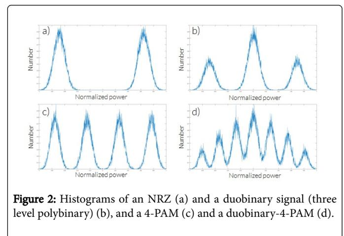
**Figure 2:** Histograms of an NRZ (a) and a duobinary signal (three level polybinary) (b), and a 4-PAM (c) and a duobinary-4-PAM (d).
