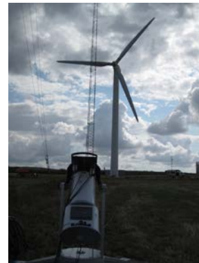
Figure 1 Picture of one of the three short range WindScanners (R2D3) deployed around the Nordtank turbine at DTU Risø Campus site.
