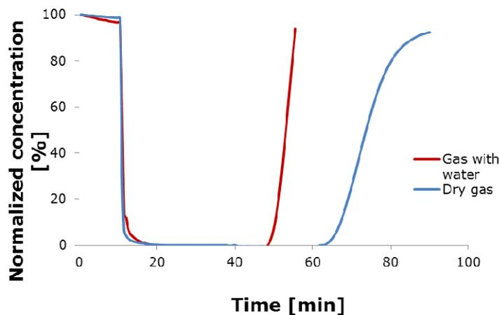
Figure 4. SO<sub>2</sub>-absorption by 20 wt% [TMGH]Cl-SiO<sub>2</sub> SILP absorber in dry 0.15 % SO<sub>2</sub>/N<sub>2</sub> and this gas saturated with water (3 %) until breakthrough.
