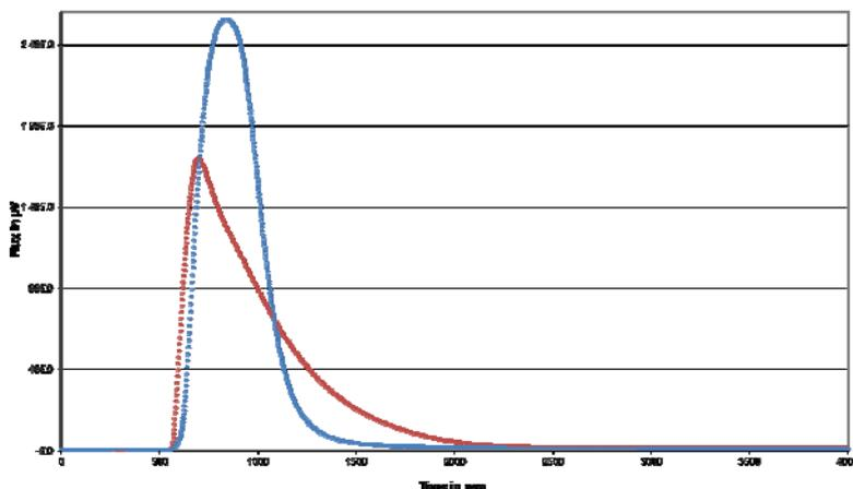
Figure 5. Thermograms (selected time period) of 1 mmol [TMGH]Cl in dry SO<sub>2</sub> (blue) and in humid SO<sub>2</sub> with 2.3 % H<sub>2</sub>O vapor (red) at 25 °C with gas flow of 5.0 ml/min.
