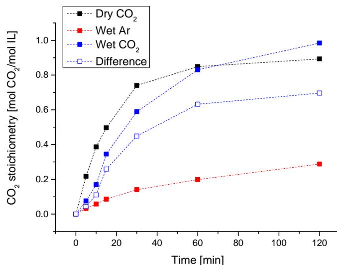
Figure 7. Uptake of CO<sub>2</sub> by dry [N6666][Pro] at room temperature during absorption in dry CO<sub>2</sub> (black), in wet Ar (red) and in wet CO<sub>2</sub> (blue, full), as well as in wet CO<sub>2</sub> corrected for mass increase in wet Ar (blue, open).
