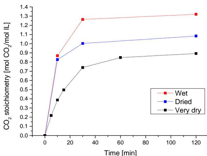
Figure 6. CO<sub>2</sub> absorption capacity in [N6666][Pro] at room temperature as a function of time with varying degrees of IL dryness (see Table II).
