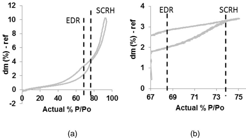
**Figure 2:** The measured mass change as a function of relative humidity at 25.0°C. The results shown in (a) were obtained from measurements performed in conjunction with a change of 1% RH per hour and in b) with a change of 0.08 % RH per hour.
