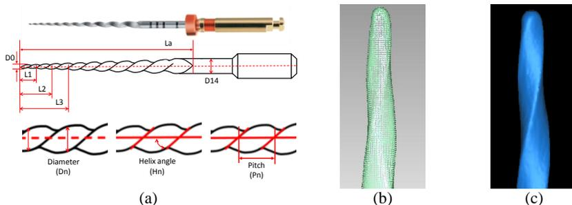
Figure 1. (a) Dental file and characteristic dimensions: length of the active cutting part ( $L_a$ ); diameter ( $D_n$ ); helix angle ( $H_n$ ); helix pitch ( $P_n$ ); (b) point cloud and (c) surface obtained from the CT scanning.
