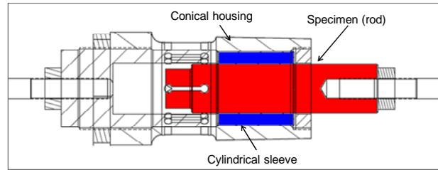
**Figure 3:** Axial section of the assembled AST rig (Strecon<sup>®</sup> container not shown).
