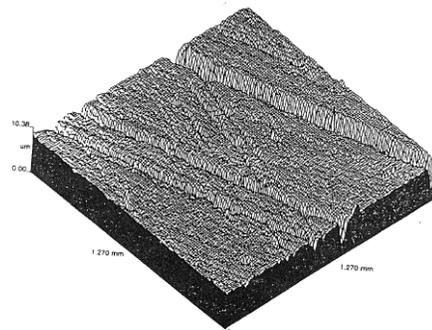
**Figure 1:** Isometric plot of a plateau-honed surface [7].
