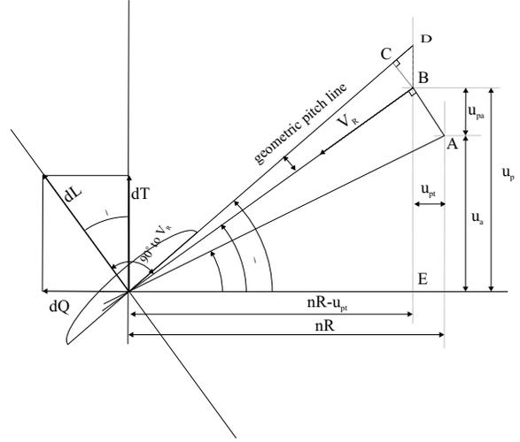
Fig. 2. Flow velocity diagram for a section of a propeller blade with rotational speed  $n$  rad/s.  $u_a$  is the undisturbed inflow velocity to the screw propeller.  $u_{pt}$  and  $u_{pa}$  are tangential and axial induced velocities.  $\beta_i$  is the hydrodynamic angle of attack and  $\alpha$  the incidence angle to the blade section. The relative velocity  $V_R$  and  $\alpha$  determine the lift force.
