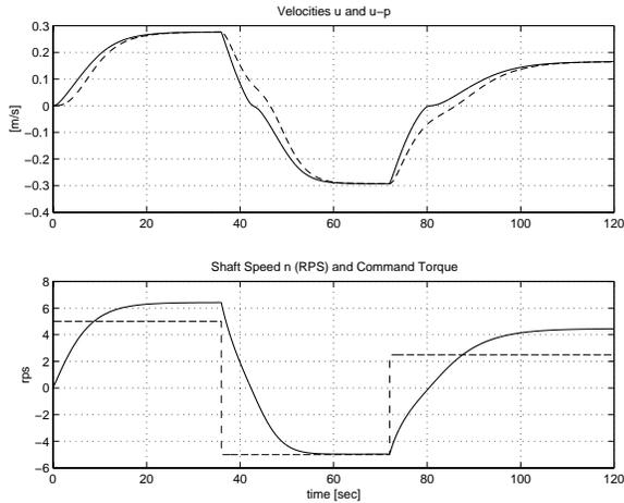
Fig. 4. Axial flow  $u_p$  (---) ship speed  $u$  (—) and propeller rotational speed  $n$  plotted over time with the test sequence applied. The  $w$  and  $a$  constants were adjusted to give easy comparison between  $u$  and  $u_p$ .
