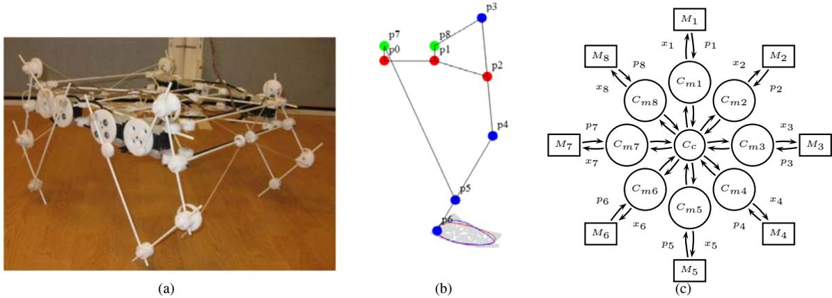
Fig. 1. (a) A quadruped robot with eight degrees of freedom constructed from the polymorphic robotic LocoKit. (b) The reachable space and two example foot trajectories are shown for the 2 DOF leg. (c) The CPG network architecture of coupled oscillators to control the LocoKit robot. The network consists of eight motors controlled by oscillators coupled to a single central oscillator.
