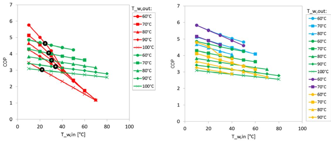
Figure 7: Left: Comparison of COP of one NH<sub>3</sub> system and one CO<sub>2</sub> system at  $T_e = 10^\circ\text{C}$  for different water outlet temperatures. The black circles mark the crossing points of the CO<sub>2</sub> and NH<sub>3</sub> systems at equal water outlet temperatures. Right: Comparison of the performance of the four different NH<sub>3</sub> systems at different water outlet temperatures and  $T_e = 10^\circ\text{C}$ .
