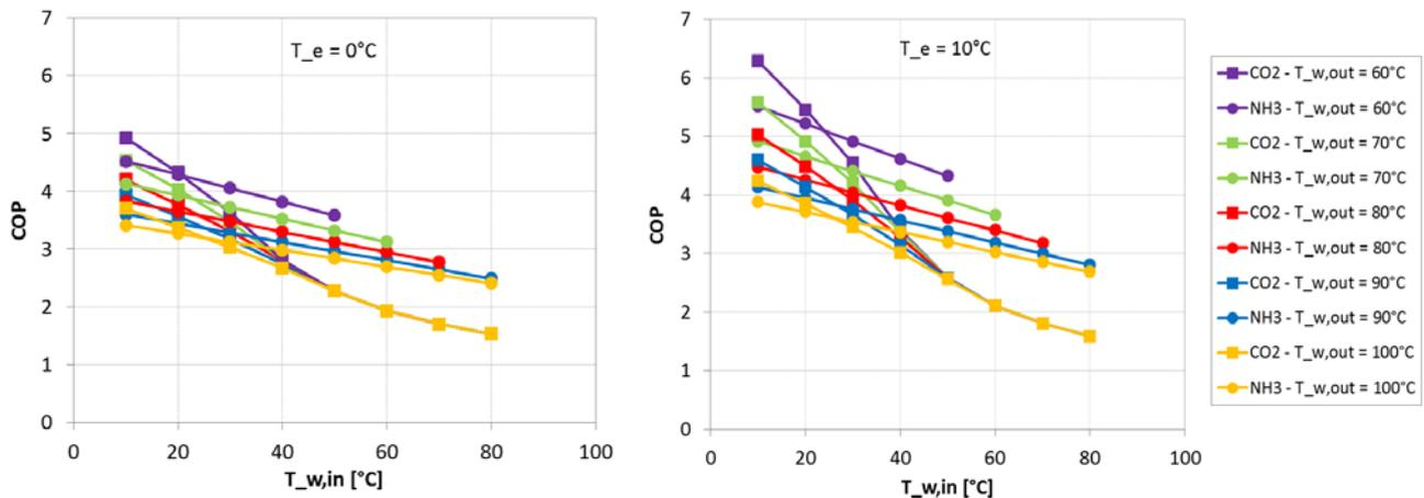
Figure 5: COP as a function of water inlet temperature for different water outlet temperatures. Results for two different evaporation temperatures are presented,  $T_e = 0^\circ\text{C}$  (left) and  $T_e = 10^\circ\text{C}$  (right).
