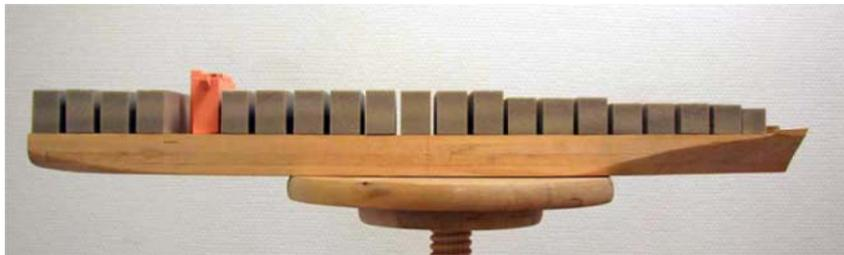
**Figure 5 - Wind tunnel model with full deck load.**
