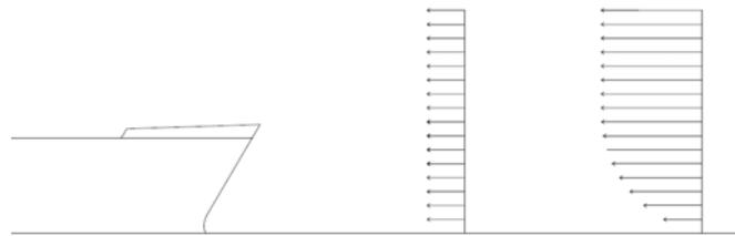
**Figure 3 - Local wind field caused by ship and the natural velocity profile at sea.**
