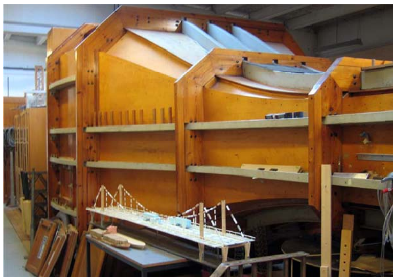
Figure 6 - Wind tunnel at FORCE Technology.
