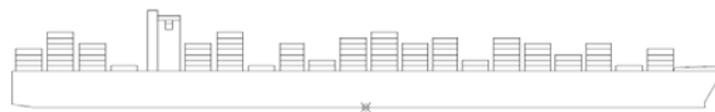
Figure 12 - Configuration 01-05-01. Random stacking over all. Highest stacking height seven containers. 68.9% of full deck stacking.
