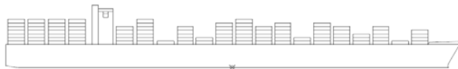
Figure 13 - Configuration 01-05-02. Random stacking fore, full stacking aft. Highest stacking height seven containers. 77.8% of full deck stacking.
