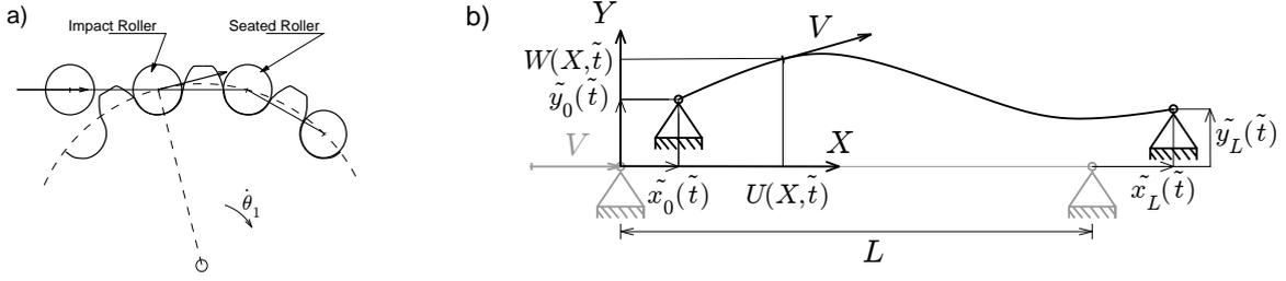
**Figure 1.** a) Meshing between chain and sprocket. The discrete nature of a chain leads to non-smooth contact between the chain roller and sprocket. b) Tensioned string traveling longitudinally between two supports moving in the plane. Shown in grey is the undeformed string moving between stationary supports.
