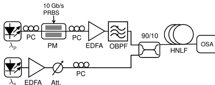
Fig. 1. Experimental setup for FOPA gain characterization.
