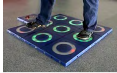
Fig.2. Modular interactive tiles used for playful physiotherapy with feet
