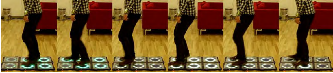
Fig.4. The scene in the playing using a wearable device and modular interactive tiles: Tiles' LED color was changed from green to yellow depending on user's HBR value.
