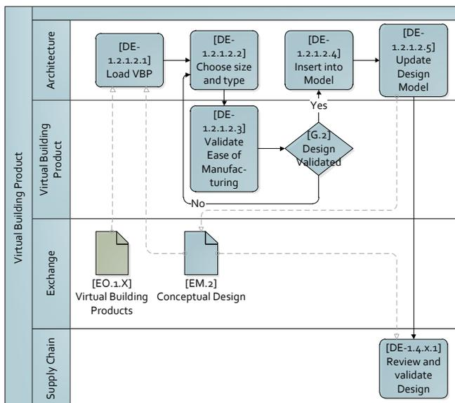
FIG. 3: Working with the Virtual Building Product
