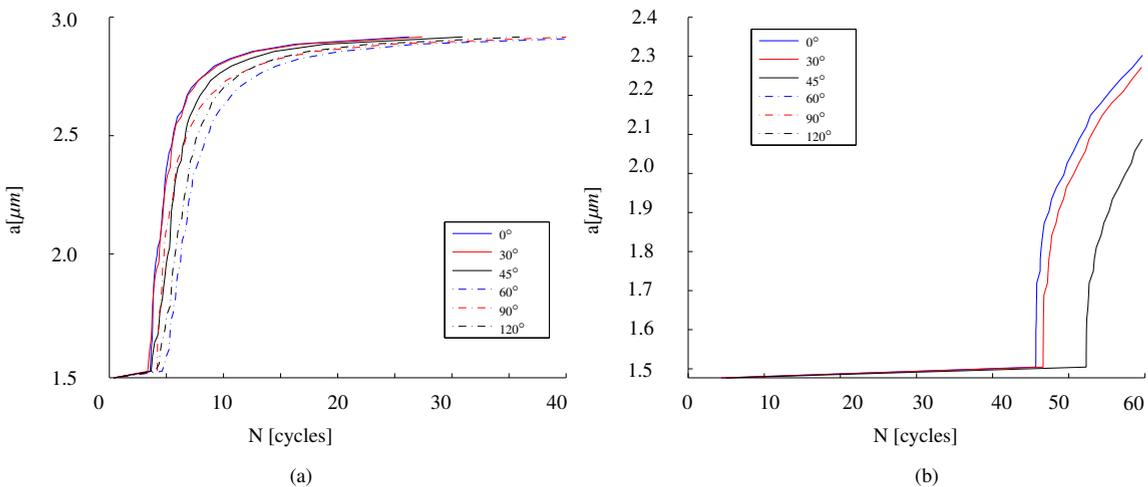
Fig. 3: Crack length evolution for ‘‘CRC’’ case, assuming (a)  $\delta_0 = 0.05 \mu\text{m}$  and (b)  $\delta_0 = 0.5 \mu\text{m}$ . In (b) only cracks with angles between  $0^\circ$  and  $45^\circ$  propagated within 60 cycles.
