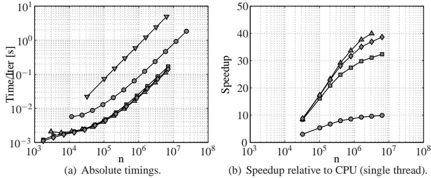
**Fig. 1** Scalability tests and performance comparisons in double precision arithmetic for Quadro FX 5800 (—●—), GeForce GTX 480 (—▲—), C2050 with ECC (—■—) and C2050 without ECC (—◆—) versus CPU (single thread) code (—▼—). Sixth order spatial discretization employed. The iterative defect correction method has been left-preconditioned with a Zebra Line Gauss-Seidel V-cycle multigrid strategy on each architecture.
