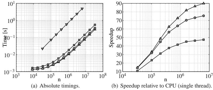
**Fig. 3** Scalability tests and performance comparisons on Tesla C2050 in single precision ( $\blacktriangle$ ), double precision ( $\blacksquare$ ), mixed precision ( $\bullet$ ), and CPU (single thread) code ( $\blacktriangledown$ ). Sixth order spatial discretization employed. The iterative defect correction method has been left-preconditioned with a Gauss-Seidel V-cycle multigrid strategy on each architecture.
