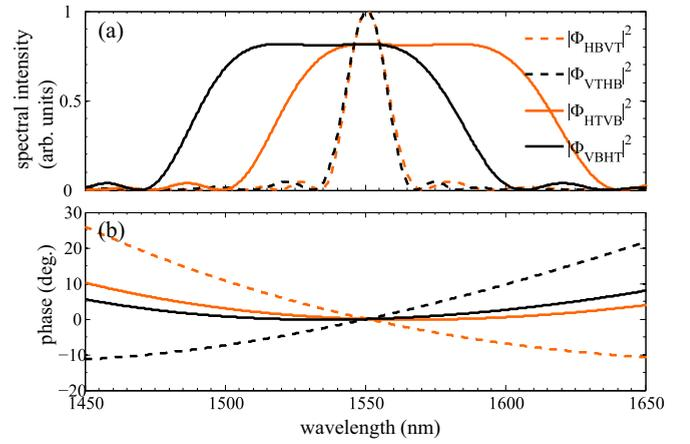
FIG. 3. (Color online) (a) Spectral intensities of the four terms in Eq. (3) and (b) the corresponding relative phases as functions of signal wavelengths using cw pump, i.e.,  $|\phi(\omega)|^2 = \delta(\omega - 2\omega_0)$ .
