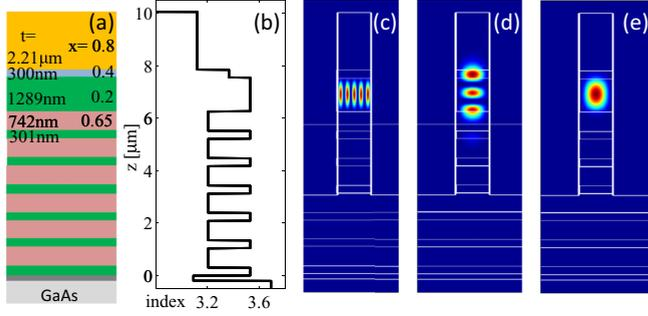
FIG. 1. (Color online) (a) Epitaxial structure of the waveguide, with layer thicknesses  $t$  and aluminum concentrations  $x$ ; (b) vertical refractive index profile at 775 nm; (c)–(e) modal intensity profiles for the pump TE<sub>40</sub> mode, down-converted TE Bragg mode, and TE TIR mode, respectively. The TM Bragg and TM TIR modes have similar profiles and are not shown here.
