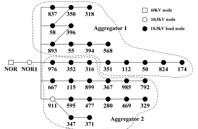
Fig. 2. Topology of the Danish 60kV/10.5kV distribution system.
