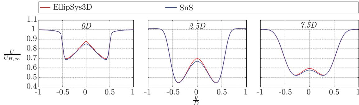
**Figure 3.** Test case one: NREL-5MW in a steady laminar uniform flow. Velocity deficit at hub height.
