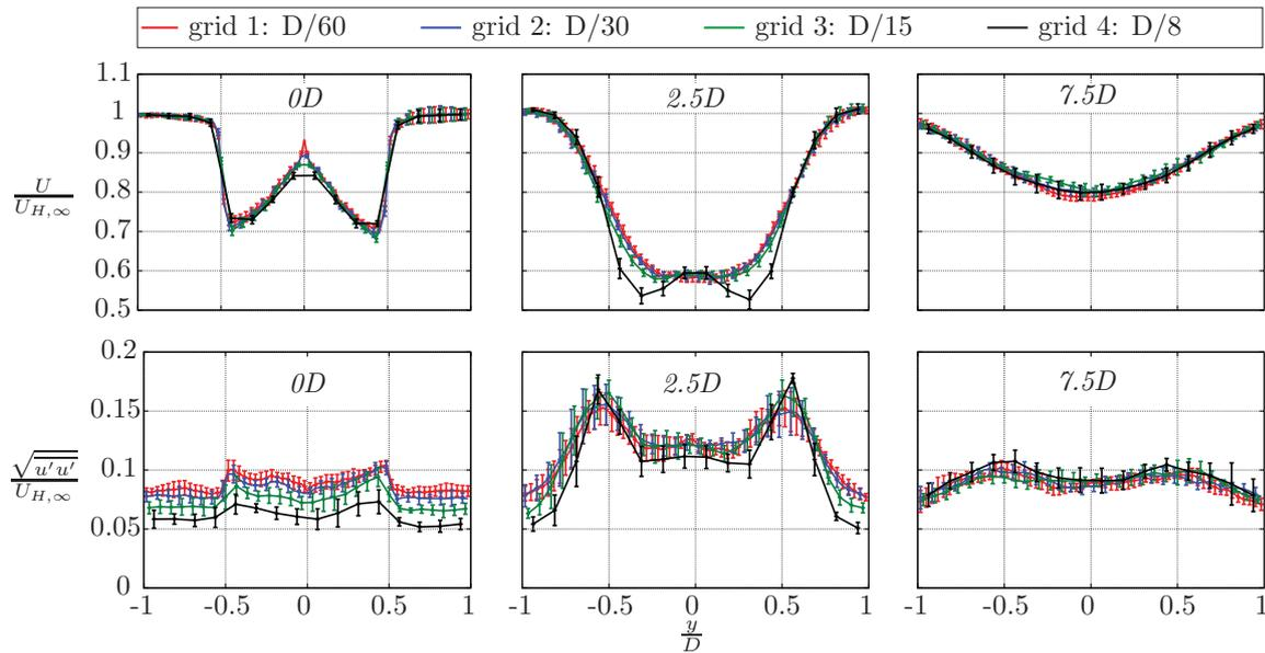
**Figure 6.** Influence of grid spacing in EllipSys3D for test case three: NREL-5MW in a turbulent uniform flow, with isotropic inflow turbulence. Velocity deficit (top) and stream-wise Reynolds-stress (bottom) at hub height.
