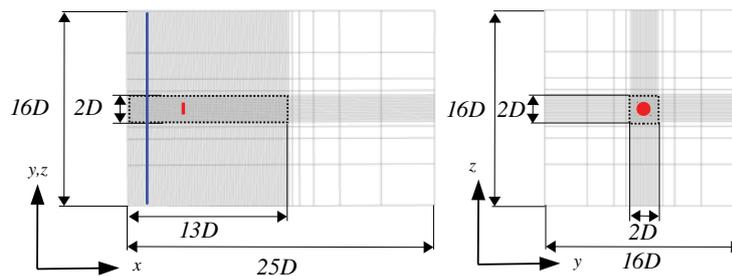
**Figure 1.** Computational domain for the uniform flow test cases. Left: side/top view. Right: front view. Dashed box marks the wake domain. AD is illustrated as a red box. Blue line represents the inflow turbulence plane. One in every four nodes is shown.
