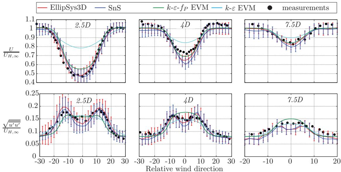
**Figure 8.** Test case four: Nibe B in a turbulent ABL. Velocity deficit (top) and stream-wise Reynolds-stress (bottom) at hub height.
