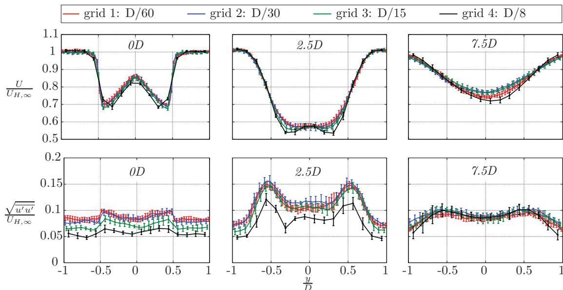
**Figure 7.** Influence of grid spacing in SnS for test case three: NREL-5MW in a turbulent uniform flow, with isotropic inflow turbulence. Velocity deficit (top) and stream-wise Reynolds-stress (bottom) at hub height.
