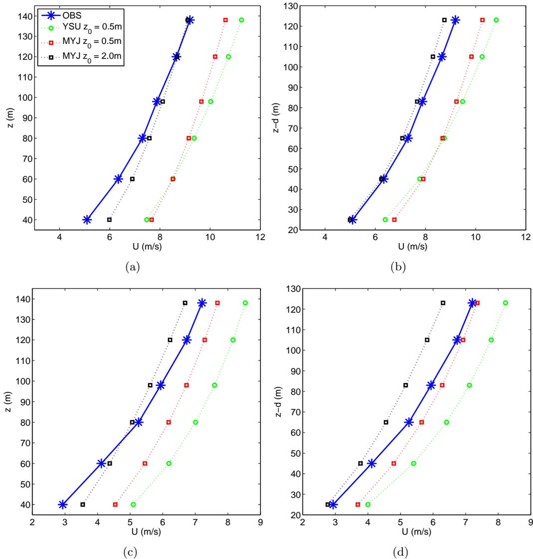
**Figure 2.** Comparison between observed and simulated wind speeds for the cases: (a) near-neutral with  $d = 0$  m, (b) near-neutral with  $d = 15$  m, (c) stable with  $d = 0$  m and (d) stable with  $d = 15$  m.
