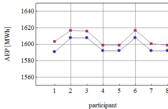
**Figure 2.** AEP with Rayleigh distribution and an annual mean wind speed of 8m/s for hub height power curve in blue and REWS power curve in red.
