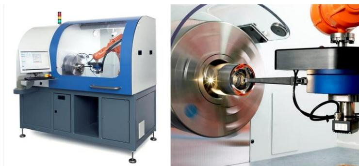
*Figure 1; STRECON's Robot Assisted Polishing (RAP<sup>®</sup>) machine tool (left) and polishing module with oscillating tool motion close up (right) (Pilný et al. 2013).*
