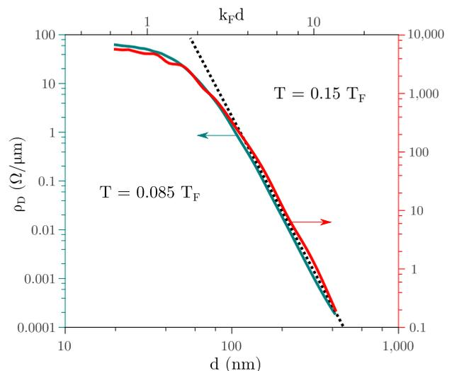
FIG. 4. (Color online) Drag resistivity between two identical ( $W_1 = W_2 = 20$  nm) GWGs as a function of distance  $d$  between them calculated at  $T = 0.085T_F$  (green line, left axis) and  $T = 0.15T_F$  (red line, right axis). The Fermi temperature is  $T_F = 580$  K and  $k_F = 0.0318$  1/nm. The black dotted line illustrates asymptotic behavior in the regime  $k_F d > 1$ .
