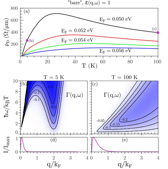
FIG. 2. (Color online) (a) Drag resistivity between equal ballistic waveguides as a function of temperature for different chemical potentials. The width of the waveguides  $W_1 = W_2 = 20$  nm and  $d = 40$  nm. Nonlinear susceptibility at different (b)  $T = 5$  K and (c)  $T = 100$  K temperatures of the system and  $E_F = 0.050$  eV. (d), (e) Normalized drag intensity calculated using Eq. (14).
