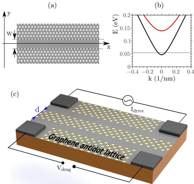
FIG. 1. (Color online) (a) Schematic illustration of a graphene waveguide (GWG): a region of pristine graphene of width  $W$  sandwiched between regions of GALs. (b) Dispersion relation of GWG with  $W = 20$  nm; the black dotted line shows a representative Fermi level  $E_F = 0.054$  eV, which corresponds to the charge density  $n \simeq 3 \times 10^{11}$  cm $^{-2}$ . (c) Coulomb drag setup: two parallel GWGs separated by the region of GAL of the width  $d$ .
