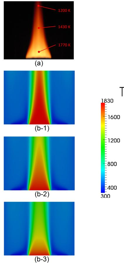
**Figure 5:** (a) picture of Helium Stabilized Rich flame [10]. (b) Contour of Flame Temperature distribution [K]: (b-1) No Radiation Modelling. (b-2) Constant Absorption/Emission Coefficient Model. (b-3) WSGGM
