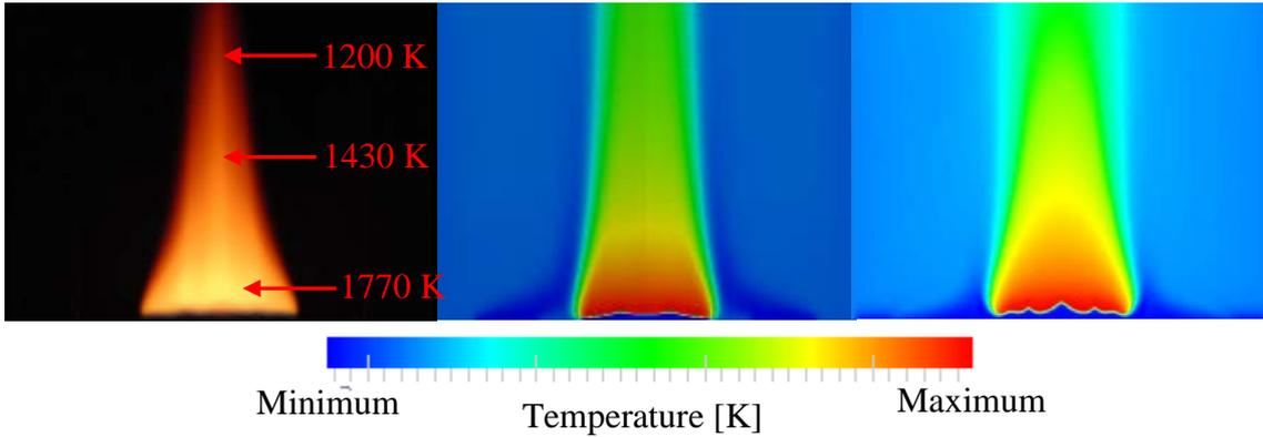
**Figure 5.** Comparisons of (a) flame images recorded from experiment against temperature contours [29] simulated by (b) OpenFOAM and (c) ANSYS CFX [29]. The minimum temperature is 300 K for both simulation cases while the maximum temperatures are 1836 K and 1810 K in the OpenFOAM and ANSYS CFX case, respectively.
