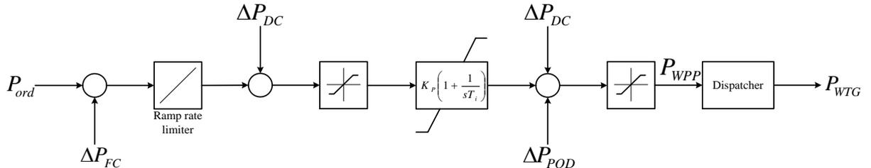
**Figure 4 - Simplified block diagram of the OWPP controller.**
