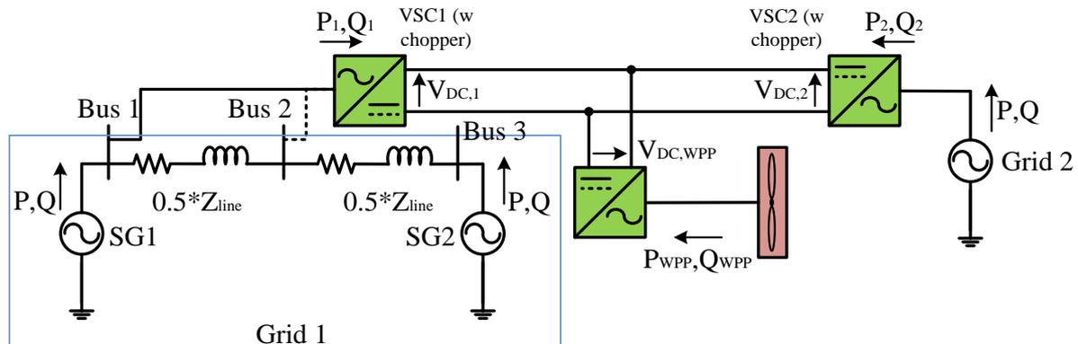
Figure 1 - Simplified simulation setup diagram.
