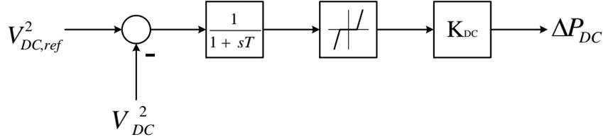
**Figure 6 - DC voltage control loop for HVDC converters and OWPP.**
