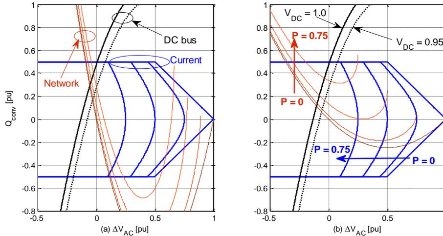
**Figure 2 - VSC capability curves and AC network characteristics in the  $Q$ - $\Delta V_{AC}$  space. (a) SCR = 5.0, (b) SCR = 1.0. All quantities are in pu of converter ratings.**
