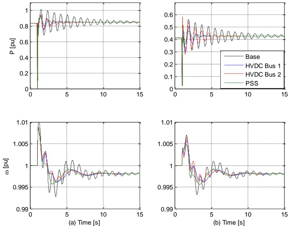
**Figure 5 - System response to excitation of power oscillations and POD contribution from HVDC network. (a) Machine SG<sub>1</sub>, (b) Machine SG<sub>2</sub>.**
