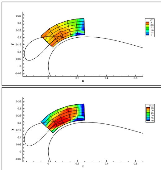
Figure 5: Parameter study of slat positioning showing contours of  $C_l$  and  $L/D$  at  $\alpha = \alpha_{C_{l-max}} - 5$ .
