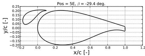
Figure 2: Optimized multiple element airfoil configuration .
