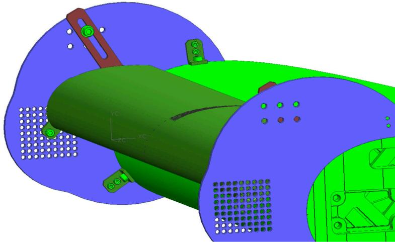
Figure 6: CAD drawing of the wind tunnel slat mounting designed by LM Wind Power.
